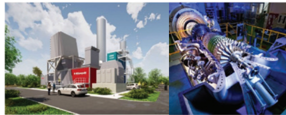
Concept of RWE's and Kawasaki's hydrogen-to-power plant in Lingen (left) and a Kawasaki Heavy Industries hydrogen gas turbine (right) (kawasaki.com)
