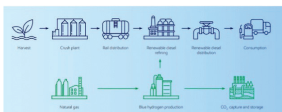
Diagram of ExxonMobil's renewable diesel production process at the Strathcona refinery (exxonmobil.com)
