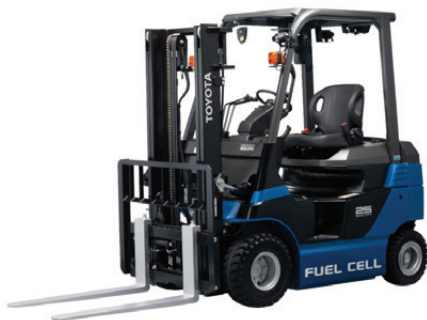
Hydrogen fuel cell forklifts by Toyota (h2-view.com)
