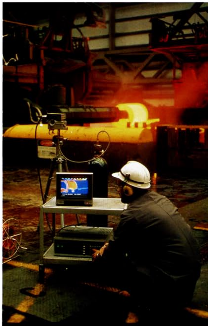
A staff member at BHP Steel's Coated Products Division, Western Port plant, uses a thermographic camera to measure heat distribution.
