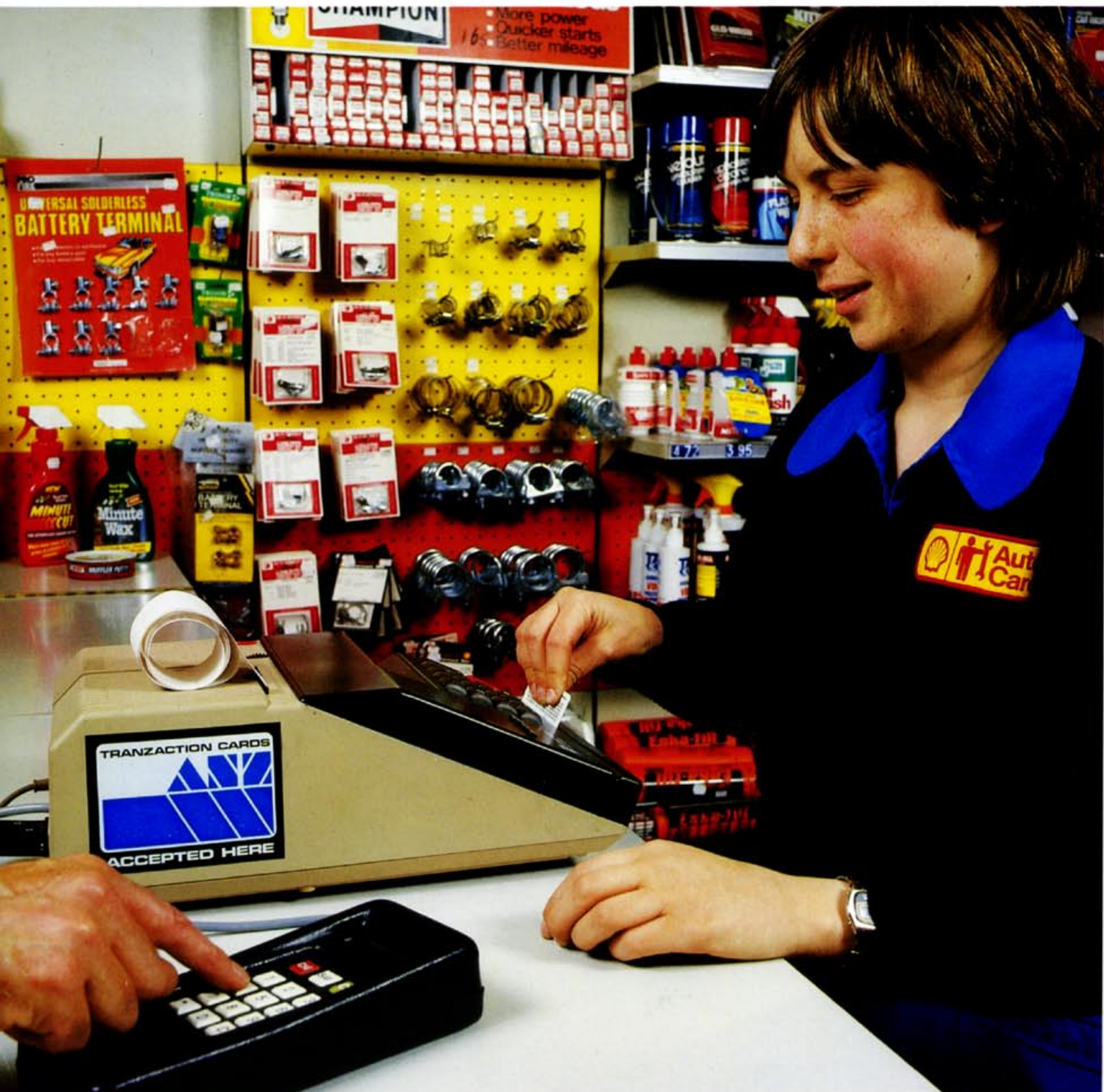
Electronic funds transfer at the point-of-sale (EFTPOS) equipment being used at a Shell service station, and providing transfer of funds within 15 seconds.
